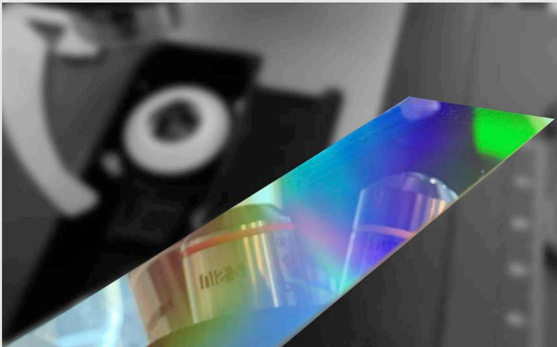
A microscope slide that can help detect cancer, developed using ANFF's NCRIS-funded nanopatterning equipment at the Melbourne Centre for Nanofabrication. Image credit: La Trobe University.
