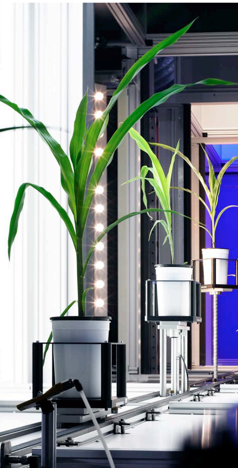
Imaging stations such as the LemnaTec Scanalyzer 3D allow for the measurement of shoot area, estimated biomass, plant height and width, canopy density, other morphometric data and leaf colour. Other sensors allow the APPF to measure a range of plant constituents, including nutrients, water or other aspects of plant physiology. Image credit: Australian Plant Phenomics Facility
