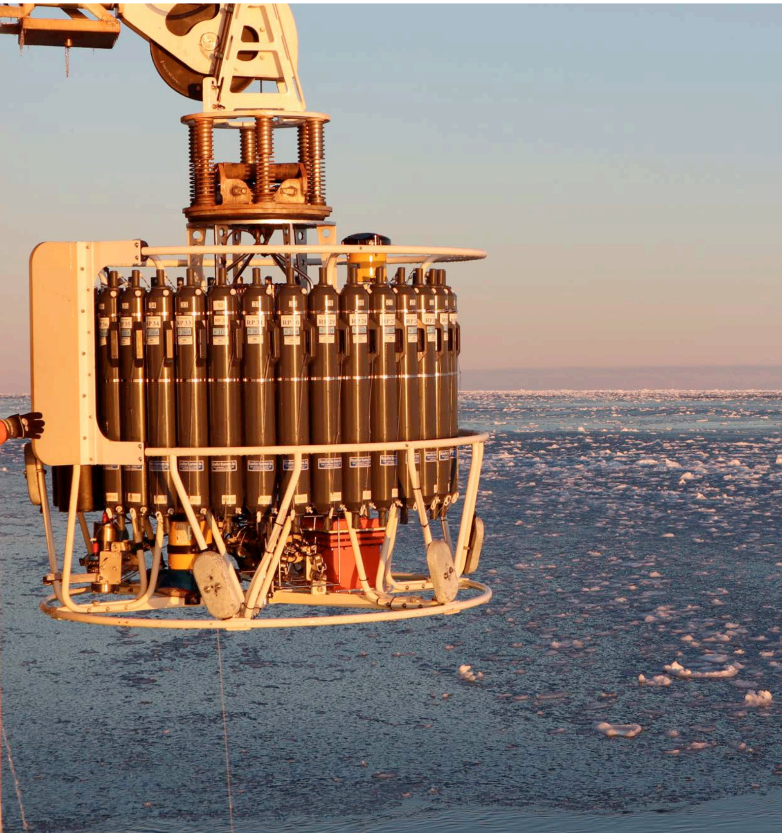
A CTD-rosette is recovered from Antarctic waters by CSIRO research vessel Investigator . Image credit: CSIRO/Merinda McMahon
